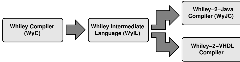
Figure 3. Illustrating the compilation pipeline.
